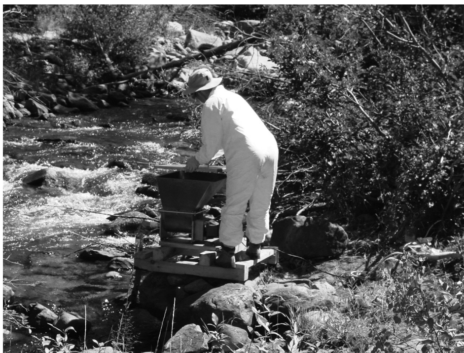
FIGURE SOP 7.3. Dispensing granular \text{KMnO}_4 into the flow of the stream with an electronically controlled auger. Once calibrated, the auger can dispense the granules at various constant rates. Note the wooden platform built out over the rocks in the flowing stream and a small gasoline generator to power the auger behind the technician.
