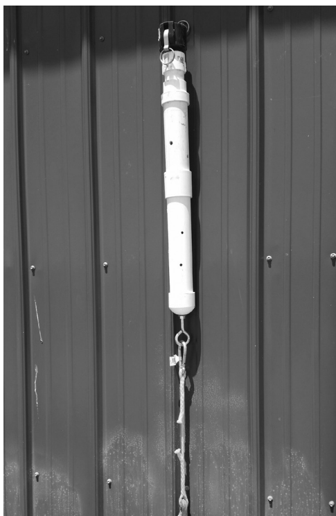
FIGURE SOP 5.2. Example of a weighted diffusion nozzle for deep-water applications.
