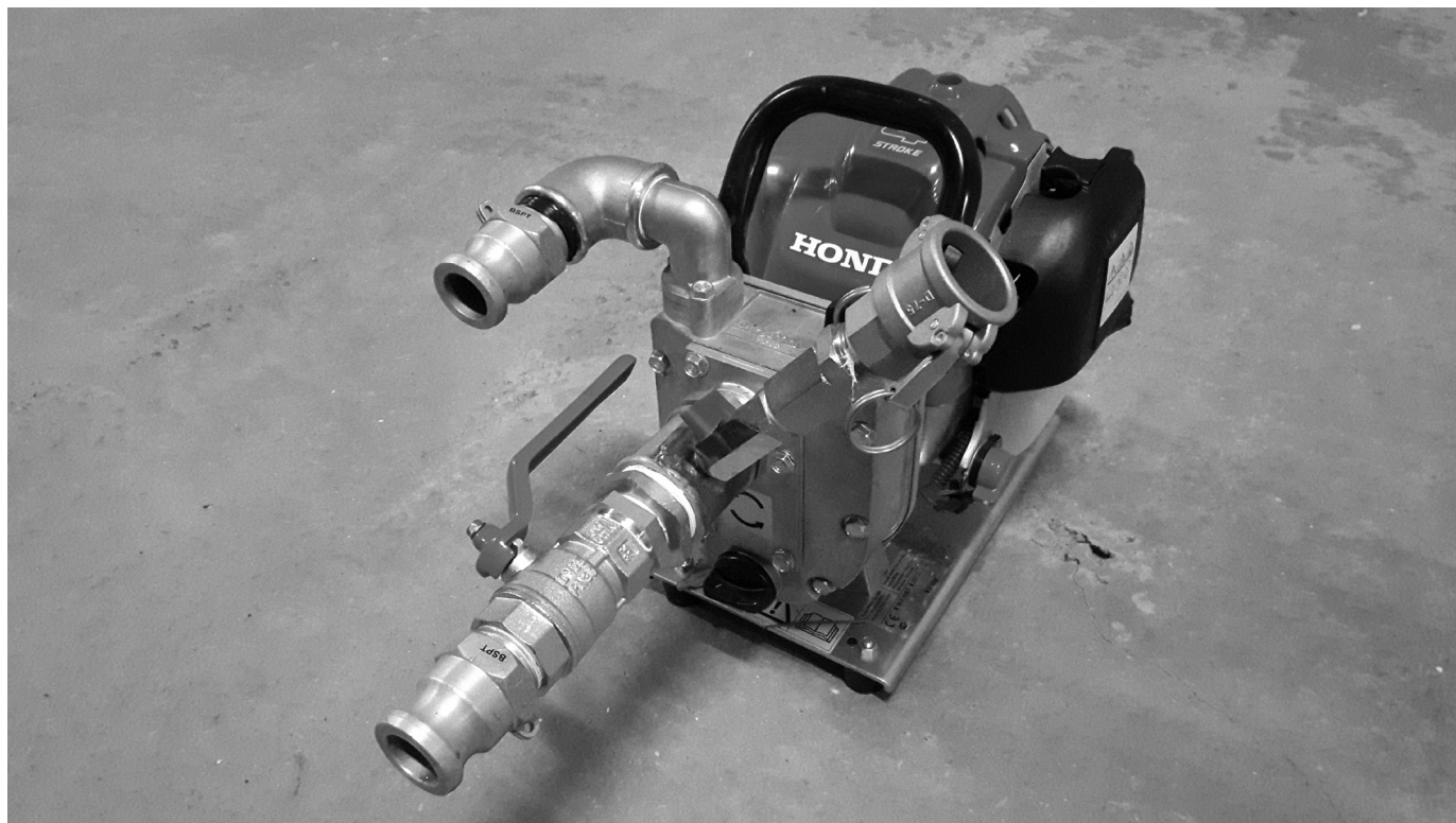
FIGURE SOP 13.1. Small portable water pump used for the application of Vectocarb/CFT Legumine slurry.
