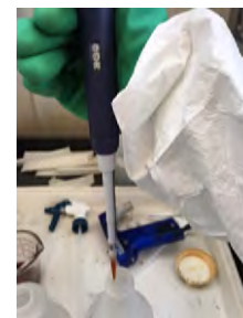
Use a safety pipette to accurately measure small quantities of liquid pesticides. Photo: C. Arrieta
