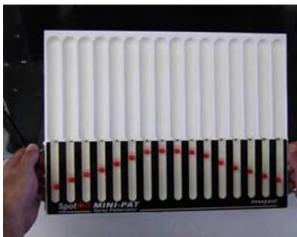
Patternator showing good nozzle pattern. Photo: Innoquestinc.com
