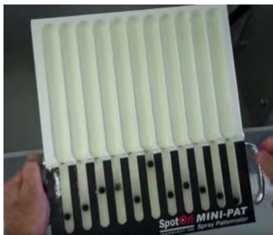
Patternator showing defective nozzle pattern. Photo: Innoquestinc.com
