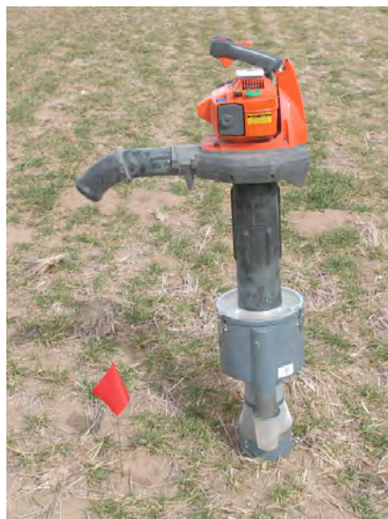
Suction sampler Image: T. Walker
