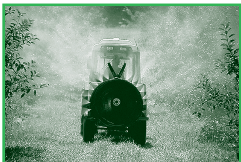
An air blast sprayer uses both water and air as carriers.
