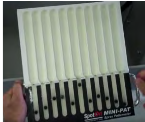
Patternator showing defective nozzle pattern. Photo: Innoquestinc.com
