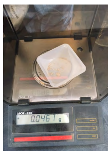
Use a scale to accurately weigh dry materials. Photo: C. Arrieta
