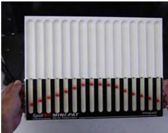
Patternator showing good nozzle pattern. Photo: Innoquestinc.com
