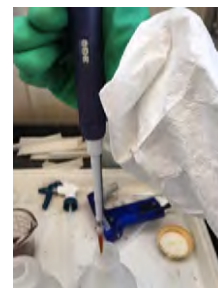
Use a safety pipette to accurately measure small quantities of liquid pesticides. Photo: C. Arrieta
