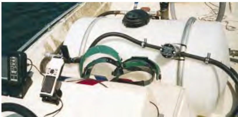
Spray boat with GPS unit, digital depth finder, digital flow meter and chemical nurse tank.
