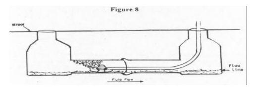
Surface coating often does not yield the results obtained by filling the pipe, since the foam is not under pressure and will not penetrate root masses as effectively as it would when filling the pipe. Repeat treatments may be necessary as succeeding "layers" of root tissue are killed off. Also, surface coating will not result in foam penetrating service connections.
