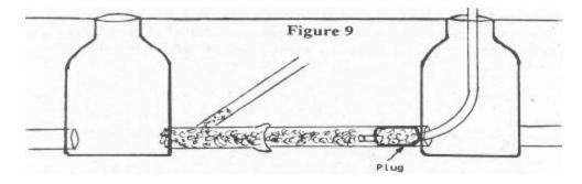
**CAUTION:** This is a high risk method. When using this method there is a <u>significant hazard</u> of foam backing into buildings, because foam will always follows the path of least resistance. This method should only be used where there are no service connections on the main-line sewer or where buildings are set far back from the main.
