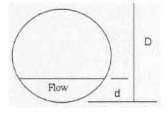
By comparing the wetted perimeter of the pipe to the entire perimeter (circumference) the applicator can determine the percent by volume of the pipe filled with water.
