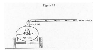
For an air-gap to be effective, the distance between the inlet line and the tank (d) must be at least twice the diameter of the inlet line (D). In the event of a reversal of pressure, air will rush through the air-gap, preventing siphoning. It is difficult to use an air gap with foaming root control chemicals, as the residual material in the tank will foam and prevent the tank from being filled.
