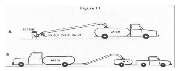
When mixing metam-sodium with water remember that metam-sodium decomposes to the more volatile and toxic MITC. This process starts immediately and proceeds rather rapidly. Therefore, plan to use the solution soon after mixing, otherwise the material will be ineffective.
