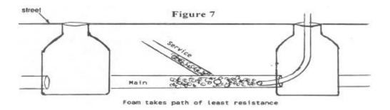
Additional foam is required per foot to use this method. Calculate the amount of additional foam required for the given number and pipe size of building laterals, and vary retrieval rates accordingly. **USE EXTREME CAUTION** to prevent foam from reaching building drains or outside sewer cleanouts.
